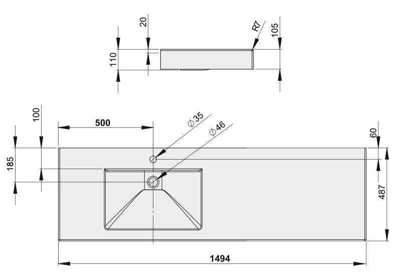
• Allowable deviation limit of product's length and width up to 1 meter: ± 5mm; over 1 meter: -5mm /+10 mm.
